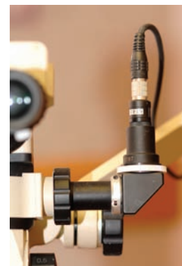
Fig. 4a: One-chip analog video camera hooked to microscope
