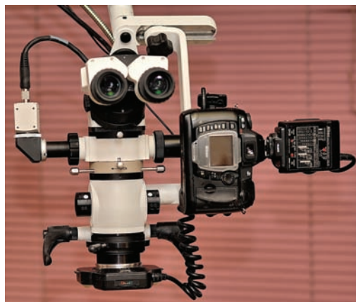
Fig. 3: Microscope with video camera (on left) and digital camera (on right)
