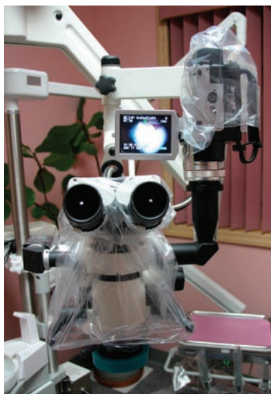
Fig. 4c: Three-chip digital cube video camera hooked to microscope
